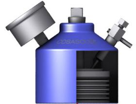
(-12) P/N 740105 Pressure Retaining Hydraulic Cover With Bleed Valve, Pressure Gauge and Center Hole for High Pressure Probe Adapter. Must use High Pressure (10,000 PSI) Probe Adapter with this Cover.
