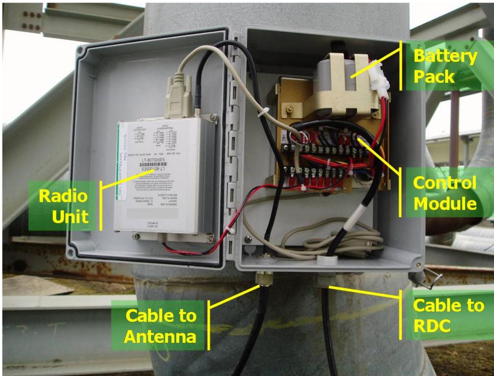
Figure 4 - Remote Monitoring Components
