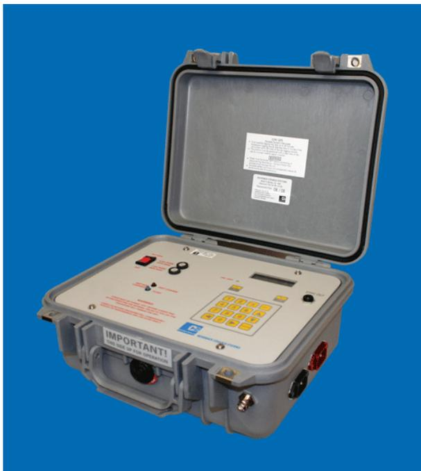
CORI-GPS Portable GPS Current Interrupter (72 dpi)
