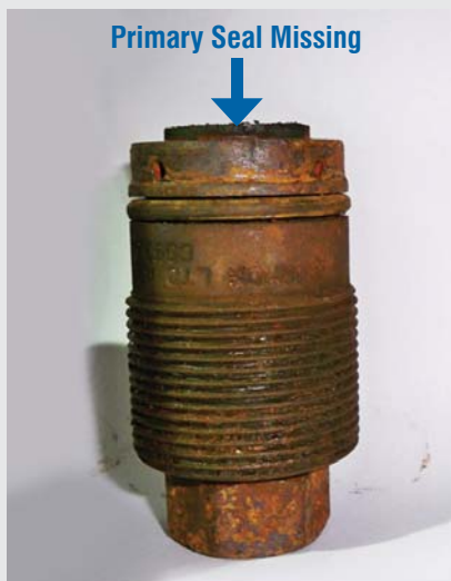
Carrier plug retrieved with no device or seal attached
