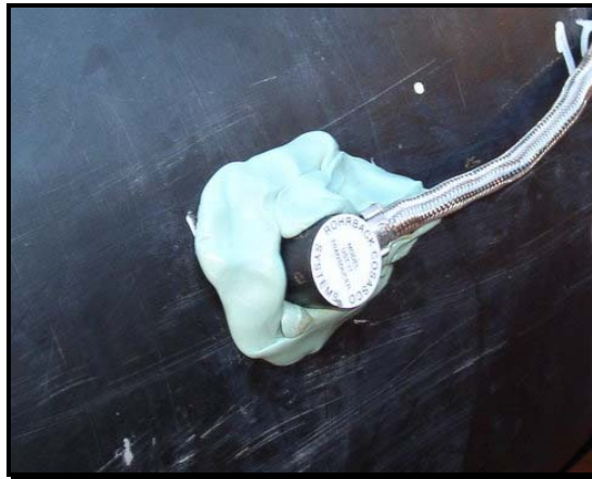
Figure 2. Mold CZ H Paste around the transducer, encasing it.
