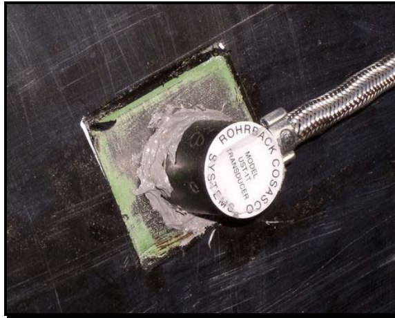
Figure 1. Let epoxy cure 24 hours after installation.
