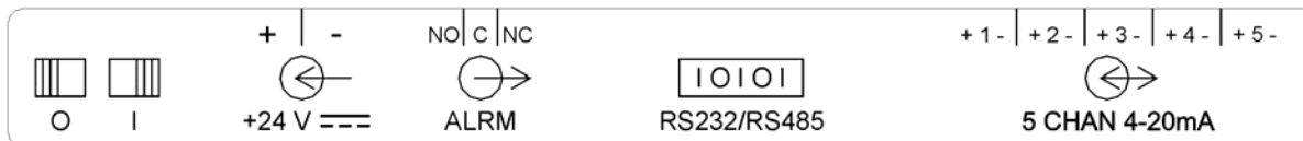
Figure 3.4 Optional Analog Outputs Located on Bottom Circuit Board
