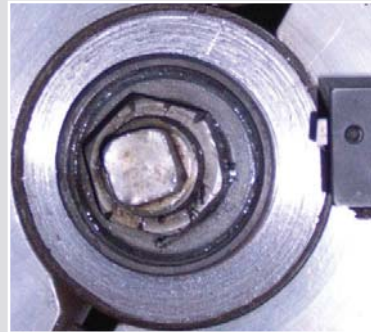
Access Fitting after re-facing
