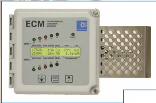
ECM™ Environmental Condition Monitor with Copper and Silver Corrosion Sensors
