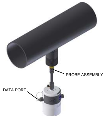
DATA-LOGGER MOUNTED ON UNDERSIDE OF PIPE
