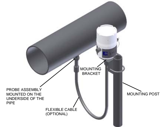
DATA-LOGGER MOUNTED IN REMOTE LOCATION
